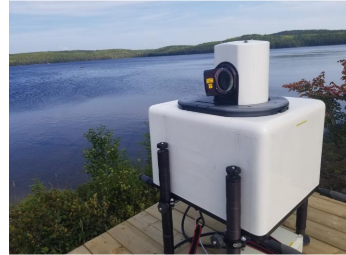
Halo lidar deployment at the Experimental Lakes Area Low-level turbulence observations over the lake boundary Collaboration with HIWR and RPN-E
